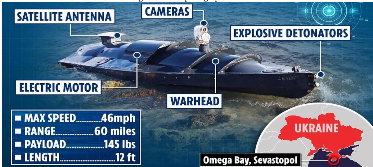
Figure 4. Same photograph, annotated
